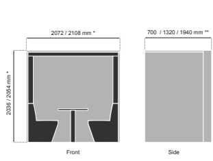
* Clad Option - 36 / 54 mm (54 mm in ply only) ** Capacity Option - 2 person / 4 person / 6 person
