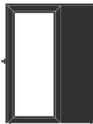
Residence Connect DDA 60"w x 45½"d x 88"h 1562w x 1156d x 2235h (mm)
